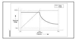
Figure 3 Torque speed characteristics of induction motor
