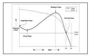
Figure 2 Torque speed characteristics of induction motor
