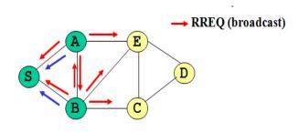
Figure2. Route Request control packet in AODV
