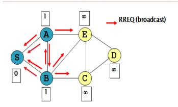
Figure4. Route Request control packet in AOMDV
