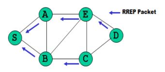
Figure3. Route Reply control packet in AODV
