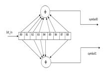
Fig.3. Proposed convolutional encoder
