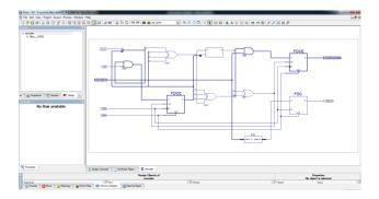
Fig.7. Internal structure of convolutional encoder
