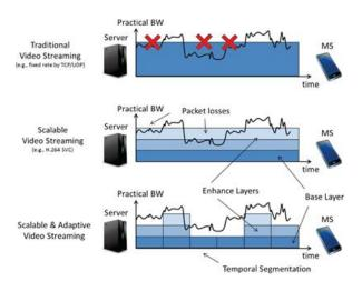
Fig. 1. A comparison of the traditional video sharing, the scalable video streaming of the VBES-Cloud framework.
