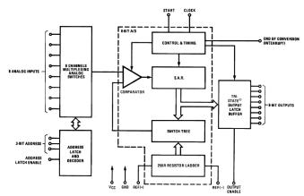
Fig. (1). Block Diagram of ADC
