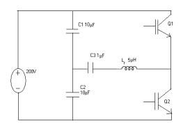
Fig.5. Zero current switching circuit
