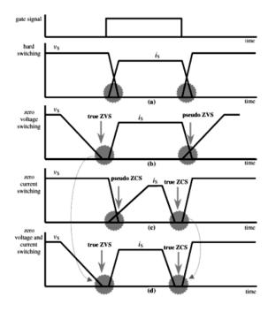
Fig.6. Comparison between switching techniques
