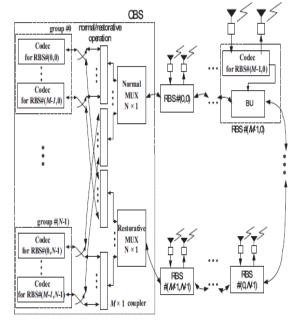
*Figure2. Fibre radio ring network*
