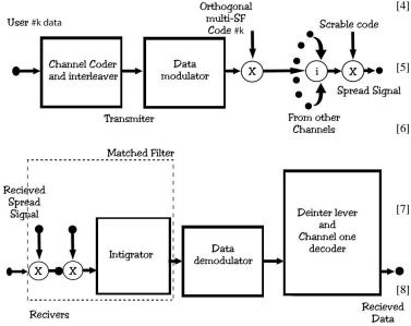
Figure 5. Orthogonal Forward Link Transmitter and Receiver Structure
