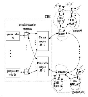
Fig. 4. The proposed fiber-radio network
