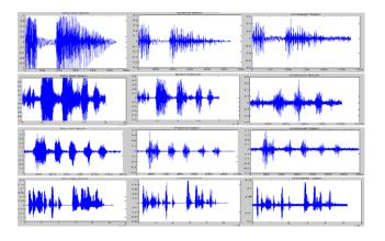
The first column presents the four different types of input signals in this noise is included and the second column presents the noise free signals which is enhanced by spectral subtraction method and the third column presents the compressed signals. compression is performed by using DWT.
