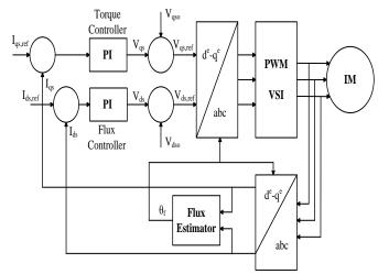
*Fig. 3 Block diagram for Indirect Field Oriented Control C. Rotor Flux Linkage Estimator*
