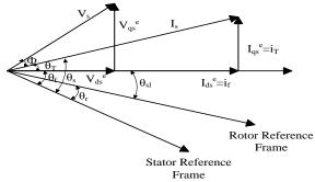
Fig. 2 Phase diagram of vector control
