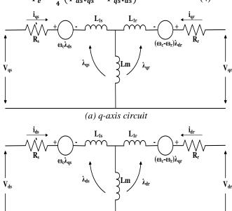
(b) d-axis circuit Fig. 1 Dynamic d-q equivalent circuits of an IM
