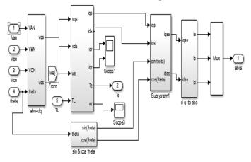
Fig. 7 Simulink Model of Induction Motor
