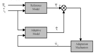
Fig. 5 Generalized model reference adaptive system
