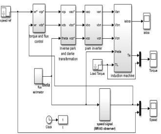
Fig. 9 Simulink Model of Indirect Field Oriented Control of IM Drive with MRAS Speed Observer
