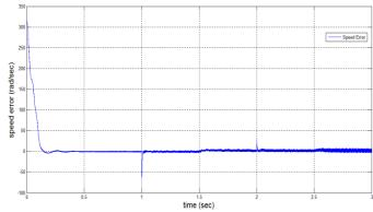
Fig. 11 speed error of the motor for changes in speed and load torque
