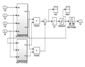
Fig. 8 Simulink Model of Rotor Flux Based MRAS Speed Observer
