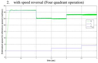
Fig. 10 Estimated and reference speed of the motor with step changes in load torque
