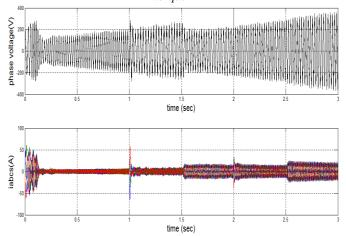
Fig. 13 Phase voltage vao and 3-ph currents of the motor with step changes in load torque
