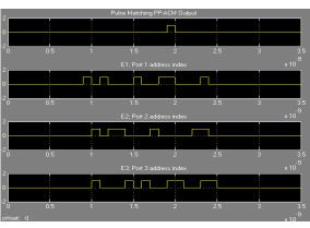
Figure 9. Output pulse of PP-ACM for matching with PPRT
