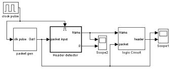
Figure 2. Simulation of header extractor in Simulink
