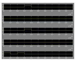
Figure 8. Output of SPC showing a<sub>3</sub>, a<sub>2</sub>, a<sub>1</sub> and a<sub>0</sub> pulses "1010"
