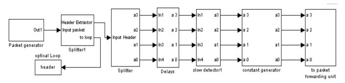
Figure 3. Packet detector and Serial-to-parallel converter
