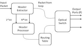
Figure 1. All-Optical Router Model
