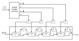
Figure 4. Pulse Position Modulation Address Conversion Module
