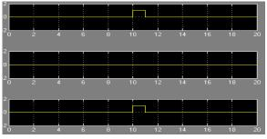
Figure 10. Two pulses generated after the match, used to drive the switch for packet forwarding
