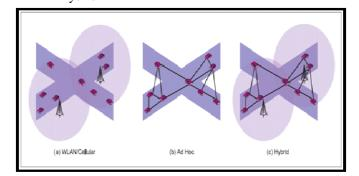
Figure 1: Three possible network architectures for VANETs.
