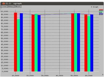
Figure 5.1: Packet delivery ratio v/s number of vehicles. *Throughput:*
