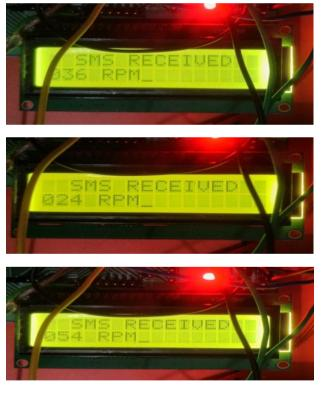
Figure 9 - Speed in RPM displayed on LCD diaplay
