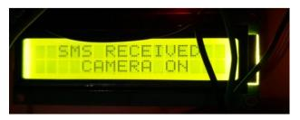
Figure 10 – Camera on message received and displayed on LCD display
