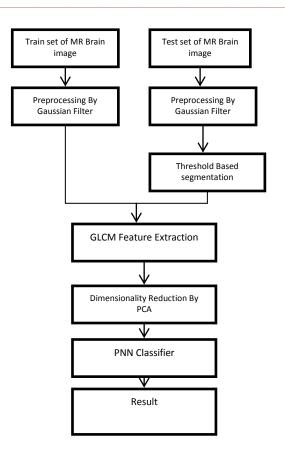
Figure 2: System Architecture
