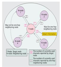
Figure 1: Detection mechanism for selfish attack
