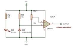
Fig. IR Sensor circuit diagram
