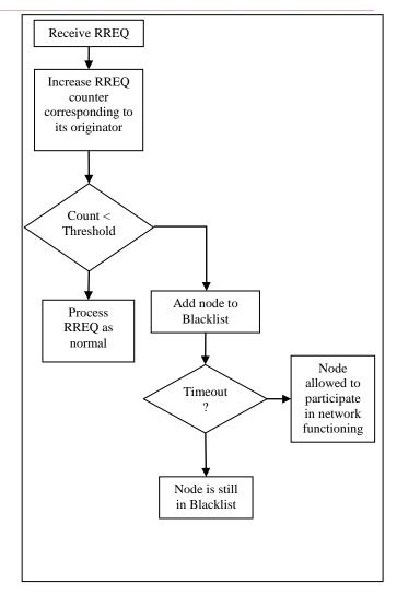
Figure 7. Modified AODV Mechanism against RREQ Flooding Attack
