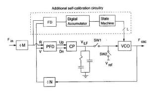
Figure 2. Self-calibrating PLL[6]
