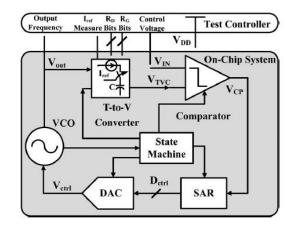
Figure 3 Self-calibrated VCO on-chip system[7]
