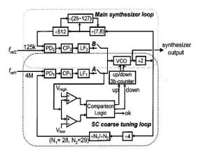
Figure 1. Frequency synthesizer schematic[5]
