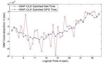
Figure 2. Generated single WAP clock delay error based on GPS time and Net- time
