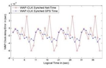
Figure 3. Generated a single WAP clock delay error based on GPS time and Net-time, and resynchronised at every 10 seconds
