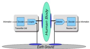
**Fig.4.1** Capacitive coupling for data transmission between transmitter and receiver units: One signal path is established through the human body while the return path has to be connected by earth ground.
