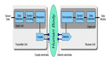
**Figure 3.1** Intra-body communication for data transmission between sensors enabled by transmitter and receiver units: The human body acts as the transmission medium.
