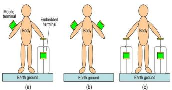
**Fig. 7.1** Typical three situations of intrabody communication. (a) Mobile embedded. (b) Mobile to mobile. (c) Embedded to embedded.
