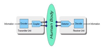
**Fig.4.2.** Data transmission by galvanic coupling between transmitter and receiver units: Differential current is coupled into the human body by the pair of coupler electrodes and sensed by the pair of detector electrodes.
