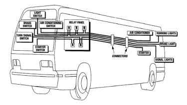
Fig.1. Conventional Vehicle Architecture
