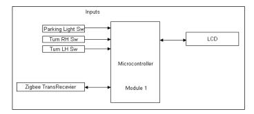
Fig.2. Block Diagram of Node
