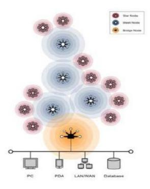
Fig.1 Wireless Mesh Network
