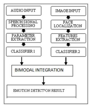
Fig. 1 flow chart of bimodal fusion for emotion detection
