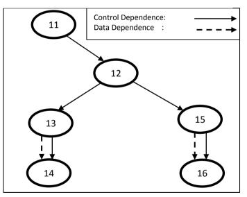
Figure-5 (SDG for aspect code of the program given in figure-1)
