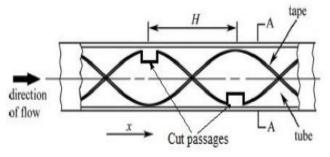
Fig.6 Construction of helical strip with regularly cut passages [6]
