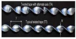
Fig.2 The Twisted tapes used in the Test Tube [2]
