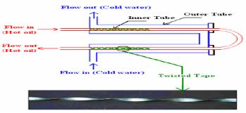
Fig. 1 Inner Tube Fitted with Half Length Twisted Tape. [1]
