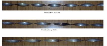
Fig 9 Reduced Width Twisted Tape (RWTT) [8]
