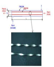
b) The inner tube fitted with twisted tape [3]
