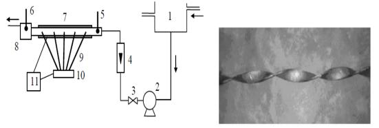
Fig. 4 Schematic Diagram of Experimental Apparatus & Twisted Tape [4]
