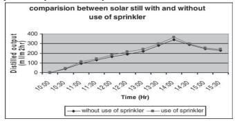
Figure 4: Use of Sprinkler in Solar Still
