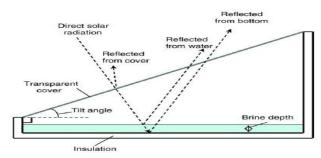
Figure 1: Schematic diagram of a basin-type solar still [1]
