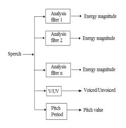
Fig.9. Channel vocoder transmitter block schematic
