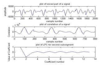
Fig. 8. Plot of LPC's for different sub-segments of Voiced segments of Speech signal
