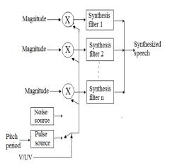
Fig. 10. Receiver for channel vocoder
