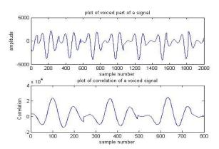
Fig. 5. Plot of Voiced part of a signal And Plot of correlation of a signal
