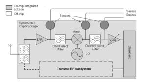
Figure 3. Sensors placed for system specification test
