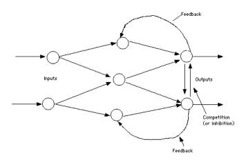
Figure 2:- Simple Network with Feedback and Competition.
