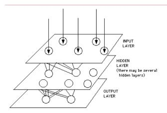
Figure 1:- A Simple Neural Network Diagram.
