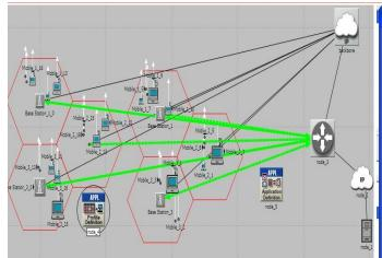
Figure 2. WiMAX Network Topology showing two Different Networks
