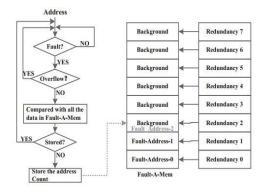
Figure 4: flows of storing fault address
