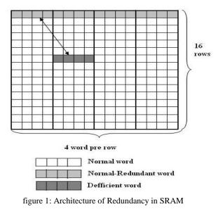
This kind of selectable redundancy architecture can save area and increase efficiency. After BISR is applied, other modules in SRAM can remain unchanged. Thus the selectable redundancy won't bring any problem to SRAM compiler.
