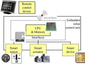
Figure 1: Embedded Robot Architecture
