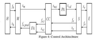
Both the assistance functions, i.e. *force assistance* (FA) and *position assistance* (PA) increase the stability and the transparency of the overall telepresence system which is beyond the degree of unassisted systems. The *force assistance* (FA) concept is valid unless the target stiffness does not exceed the value of the initial estimated stiffness. Thus the main challenge is to overcome the problem of facing a stiffness of unknown value [4].
