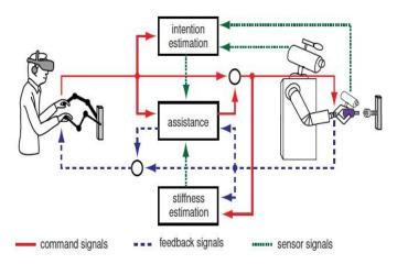
Figure 3: Concept of intelligent assistive teleoperator
