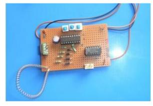
Layout of RF Transmitter Module
