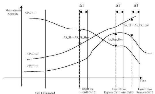
At the start of the scenario the user is connected to cell number 1 which has the strongest pilot signal. Due to the user moving or to slow fading the perception of the signal strengths to the mobile user can change and following actions are taken:
