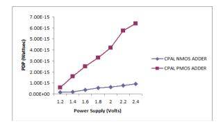
Figure 9. Comparison of PDP for the Adiabatic full adders at different supply voltages
