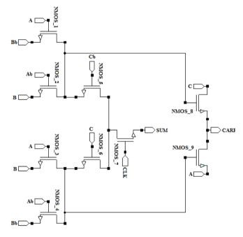
Figure 1. Proposed N-type CPAL Full Adder
