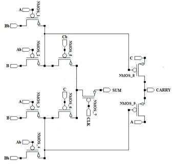
Figure 2. Proposed P-type CPAL Full Adder
