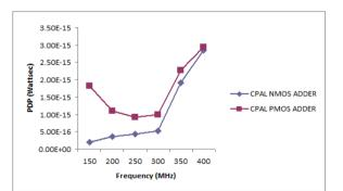
Figure 11. Comparison of PDP for the Adiabatic full adder at different operating frequencies
