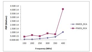
Figure 14. Comparison of PDP for the Adiabatic ripple carry adder at different operating frequencies
