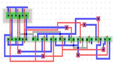
Figure 6. Layout of N-type CPAL Full Adder
