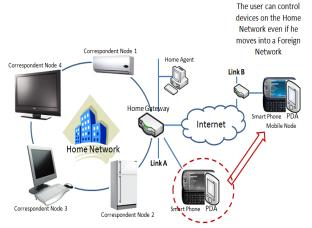
Above figure shows that user can still control the home appliances or equipments connected to the home network even if he moves into a foreign network. When the user is away from the home network ,the users mobile phone or PDA is associated with a care-of-address which identify its current location.
