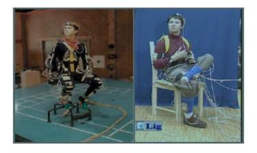
Fig- 4: Mechanical Mocap System
