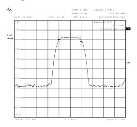
Figure15: Extracted 25 KHz Narrowband Channel
