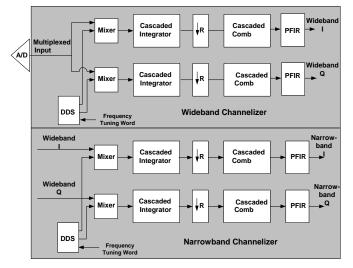
Figure 4: Wideband and Narrowband Channelizer Architecture using DDC Technique
