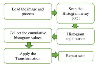
Fig.2. Block diagram of proposed method of Histogram Equailazation
