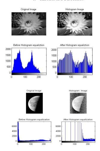
Fig.3.Simulation Results of Original and Histogram EquailizationImages
