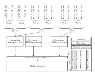
Figure. 2 Memory Organization flow for GPU Architecture.
