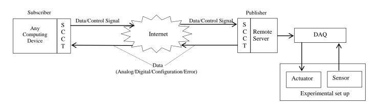
Figure 1. System Architecture of Remotely activated Virtual Laboratory
