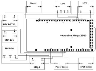
Figure 3: Circuit diagram of the proposed system.
