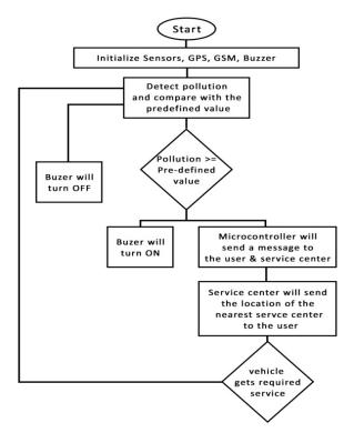
Figure 1: Flow diagram of proposed System
