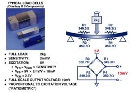
Fig 8: Typical Load Cell [28] with Sensitivity & Excitation
