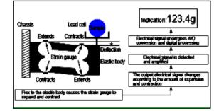
Fig 3: Load Cells in Force Sensing Structure [8]
