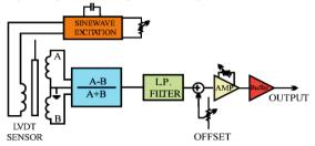
Fig 4: LVDT Based Digital Weighing System [9]
