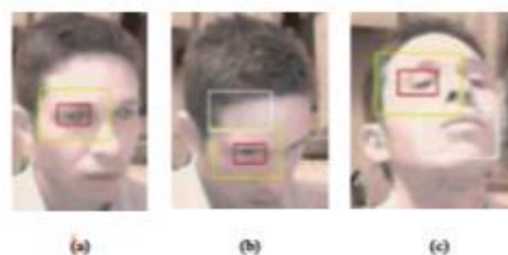
Figure 5. (a) Inner rectangle-eye area (found in the latest frame). Outer rectangle: eye search area in the present frame; (b) Inclination level of the driver's head: downward tilt; (c) Inclination level of the driver's head: upward tilt [11]
