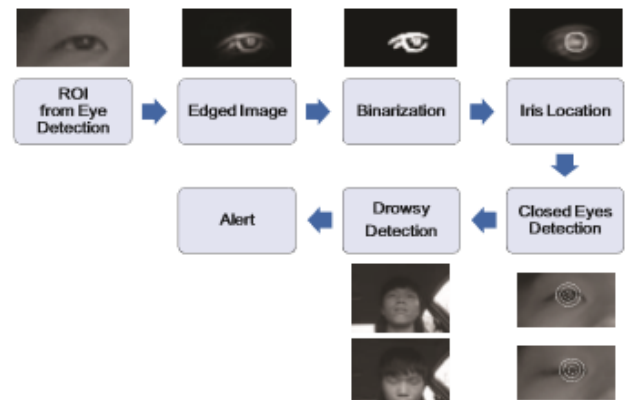
Fig. 2 Flow of the proposed drowsy driver detection
