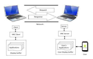
Figure: Existing system architecture
