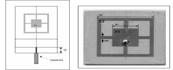
Fig.3.10 Configuration of the dual band patch
