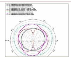
Fig.3.11 2D Polar Plot for dual band antenna 1
