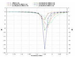
Fig.3.4. Return Loss curve for different feed points
