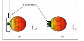
Fig 3.2 (a) 3D view of radiation pattern for cellular phone orientation in the YZ plane (b) 3D view of radiation pattern for cellular phone orientation in the XZ plane
