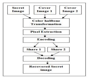
Fig 1. Block Diagram of Extended Visual Cryptography
