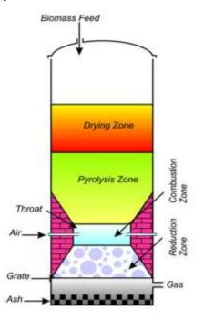
Figure 2. Schematic diagram of a downdraft gasifier
