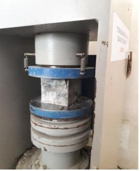
Fig c: Compression Testing machine
