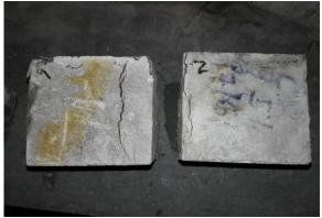
Fig b: 5% Crumb rubber concrete after compression test.
