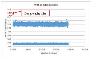
Figure 3: Clock tick processing duration of the bare-machine
