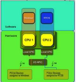
Figure 11: The procedure of configuring interrupts through the RTS hypervisor.
