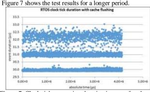
Figure 7: Clock tick processing duration in case of cache flushing
