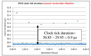
Figure 2: Clock tick processing duration of the bare-machinezoomed
