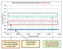
Figure 6: Clock tick processing duration zoomed version of the results on the bare-machine
