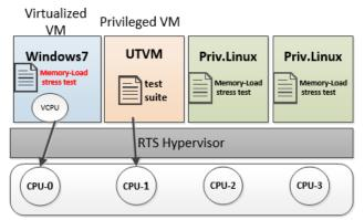
Figure 14: Scenario 3 with three VMs executing memory-load stress test
