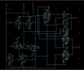
Figure 6: Logic Circuit Of Carry Block
